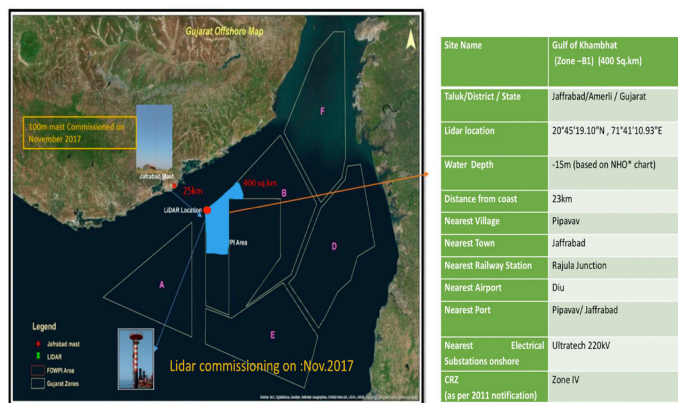
Figure 1, Information on the area offered under MNRE's tender for India's first 1GW offshore wind project
